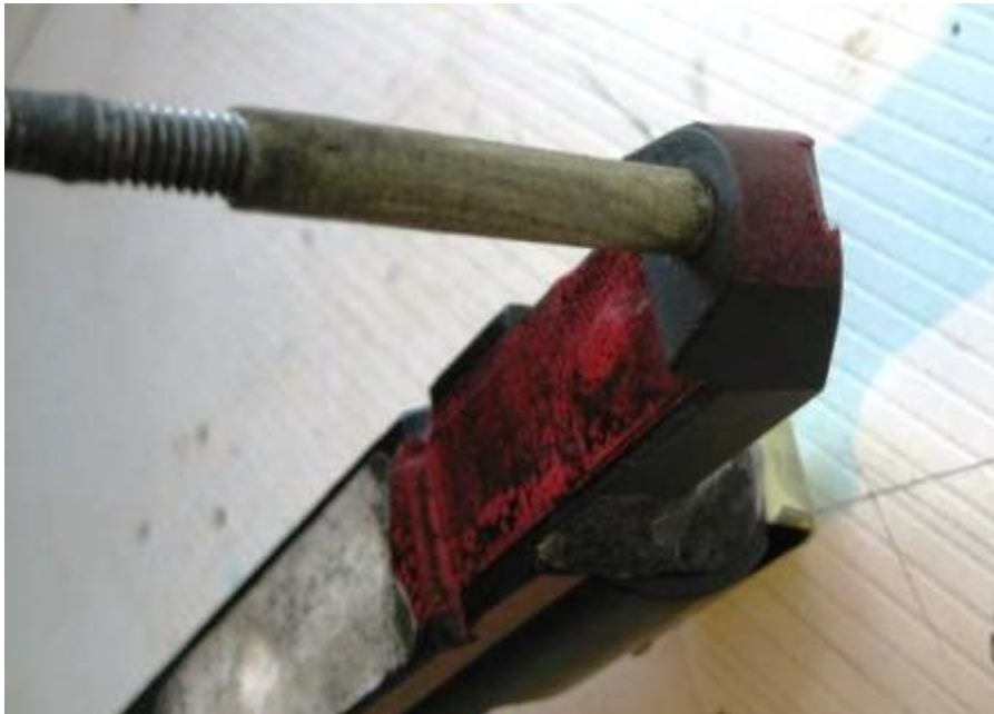
Howa wood blue rifle being prepared for bedding. Electrical tape is used for relieving, plastercine is used to plug the mag well (this rifle was full length bedded). The black release agent has been applied to the action and can be seen on the electrical tape.
