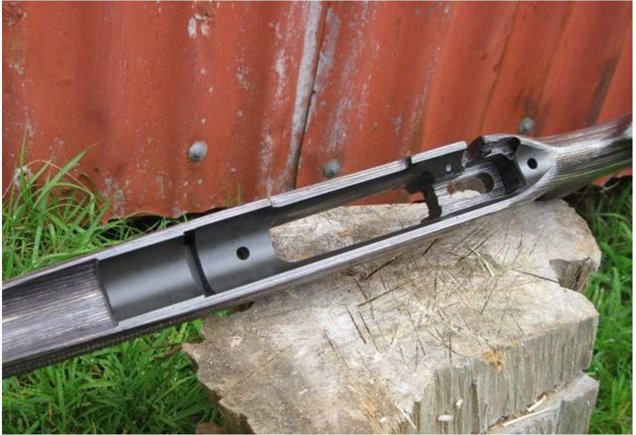
The end result. Remington M700 full length bedding
