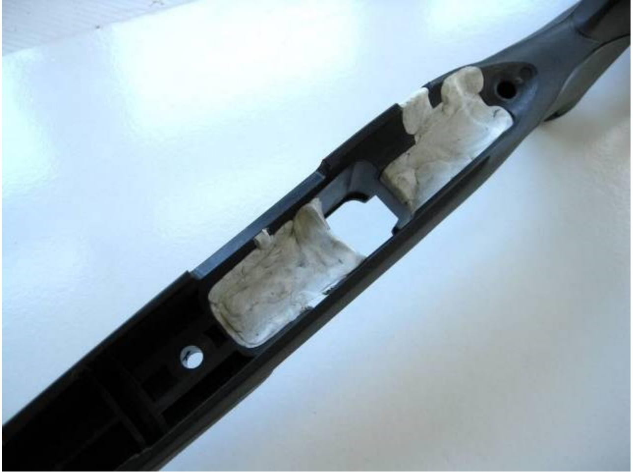
Full view of M700 stock (example) with tang dam.
